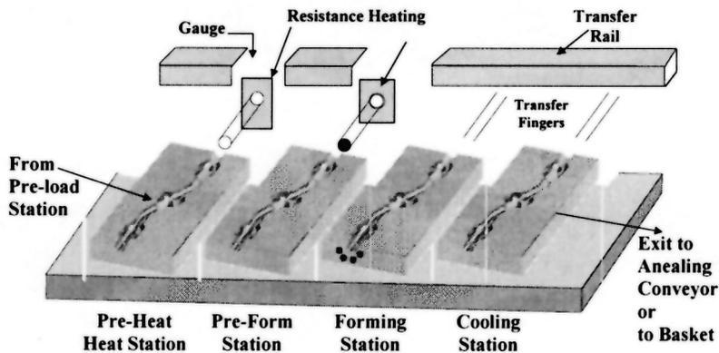
4. The pre-heated blank is placed into the HMGF station in the die. The tube receives a secondary heating to the forming temperature (about 1800 Deg F). The tools have imbedded induction-heating coils. The part end openings are sealed and the blank is expanded utilizing gas pressure (300 to 1000 psi) to expand the tube and thus fill the tooling cavity
