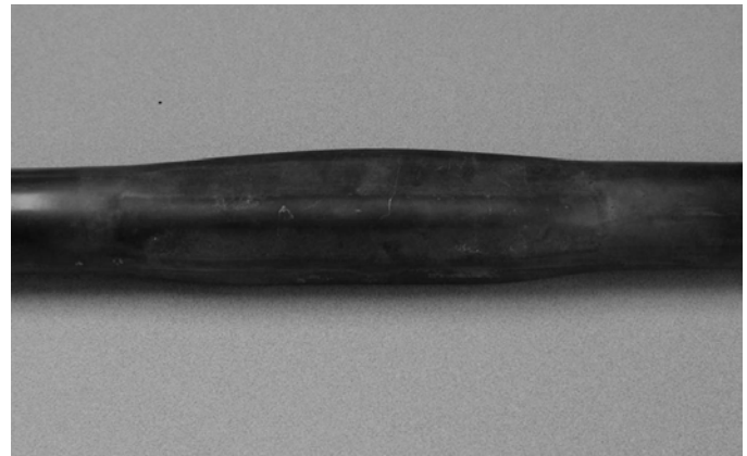
Steel part formed into a semi-square shape
