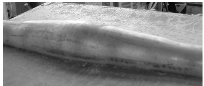
First part – Al 6061 die formed 2 to 3 diameter
