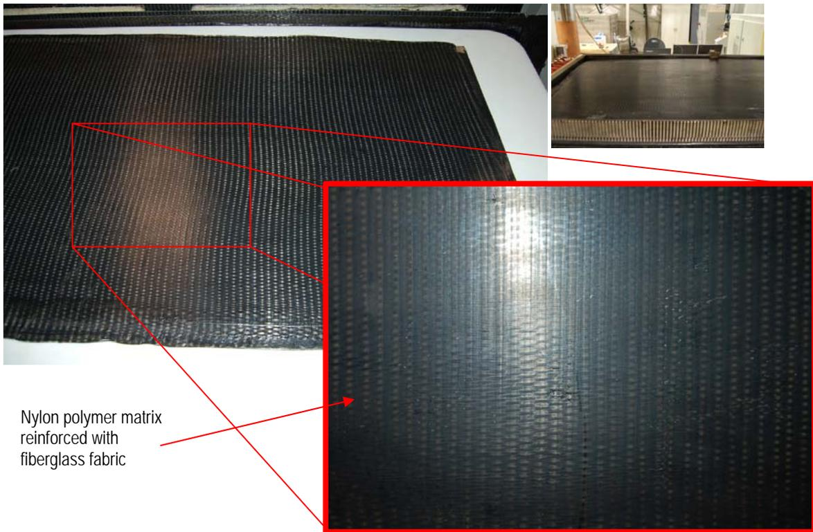
Figure 66. Picture of the as molded panel in the tool top right and then typical molded panel appear as shown in the remaining 2 pictures
