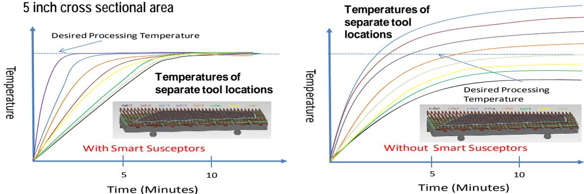
Figure 28. Depiction of the effect of the use of smart susceptors (see chart on the left) on large coils having multiple coils connected in parallel as opposed to no smart susceptors (see chart on the right)
