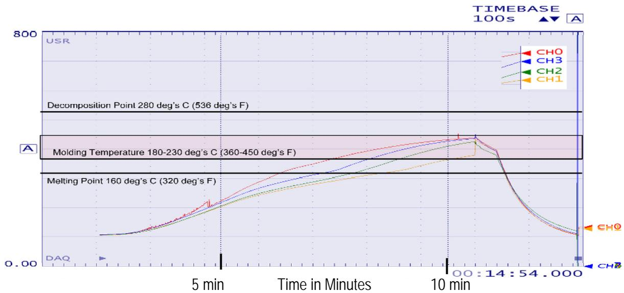
Figure 77. Temperature versus time plot for the preform during the induction molding of the Ford seat pan component
