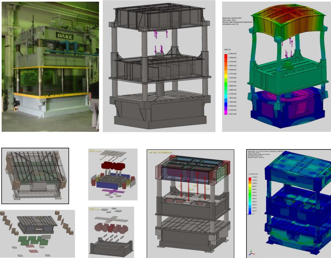
Figure 37. Picture of the used DAKE press as purchased and depictions of the subsequent analysis and redesign of the structure of the press
