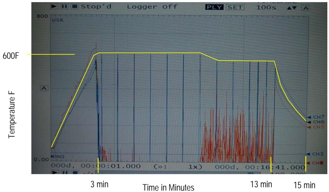
Figure 65. Typical thermal cycle for tooling surface (15 minutes) associated with the consolidation of the fiberglass/nylon 6-6 fabric laminates with the soak time associated with conduction of thermal energy into the preform
