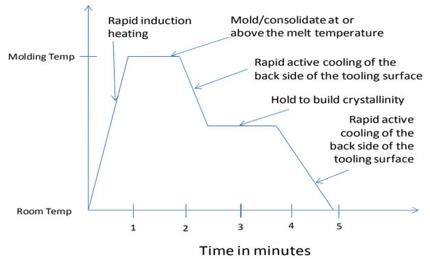
Figure 54. Picture of the typical consolidated component and the thermal cycle goal establish at the beginning of the project for the PEKK materials
