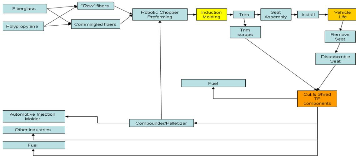
Figure 97. Direct (in automotive) recycling stream within automotive production boundary
