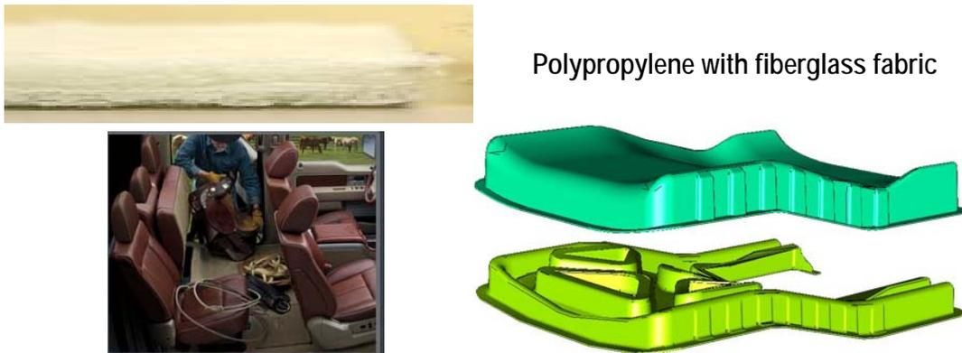
Figure 36. Depiction of Ford seat pan demonstration part for evaluation of the induction molding of random matte fiberglass reinforced polypropylene for application to automotive applications
