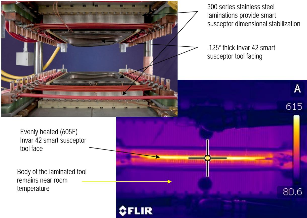
Figure 5. Typical induction consolidation tooling design on the left and then on the right an infrared picture of the tooling in operation showing the even heating of just the smart susceptor with the body of the tool remaining near room temperature
