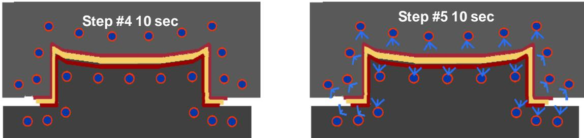
Figure 33. Depiction of the rapid molding of the preheated preform using the preheated mold with a subsequent water quench
