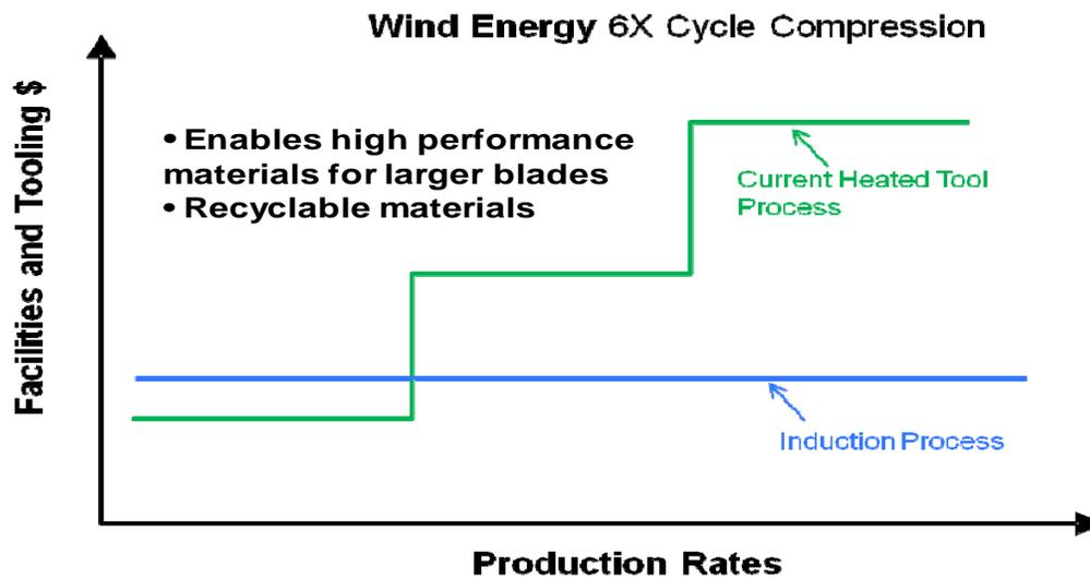
Figure 103. Chart depicting the effect of the more rapid thermal cycle on the ability to lower production costs as wind turbine production rates rise
