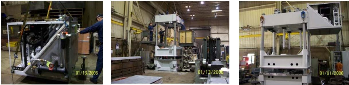
Figure 39. Pictures of the assembly of the refurbished components of the redesigned press
