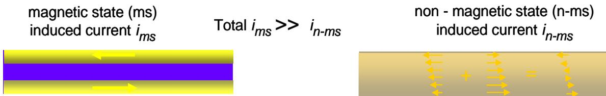
Figure 2. Depictions of the induced current distributions in the smart susceptor, with the magnetic state shown on the left and the non-magnetic state shown on the right
