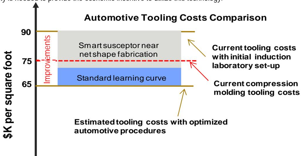
Figure 104. Chart depicting the current cost of the induction consolidation tooling to the existing compression molding tooling cost plus the estimated tool cost for the optimized induction process
