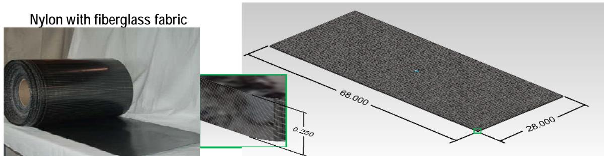
Figure 35. Depiction of Vestas flat panel demonstration panel to enable evaluation of the consolidated fiberglass/nylon materials for application to wind energy
