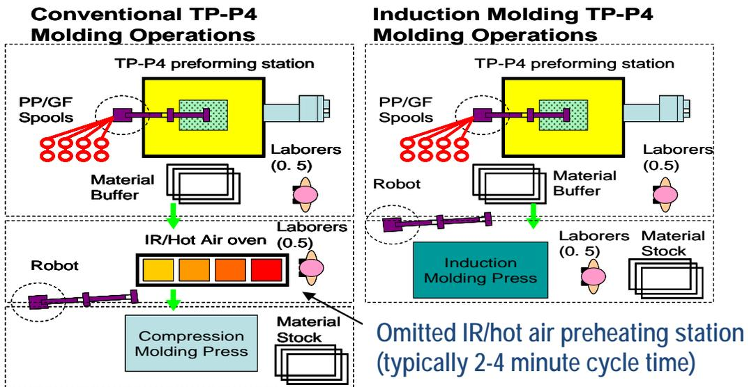
Figure 90. Diagram of manufacturing cell for the standard compression molding process for automotive applications as compared to an induction molding cell
