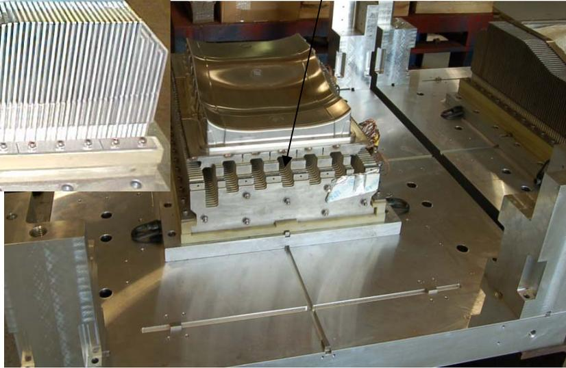
Figure 72. Completed tooling insert as shown in the upper left picture and the insert positioned on the die shown in the bottom right
