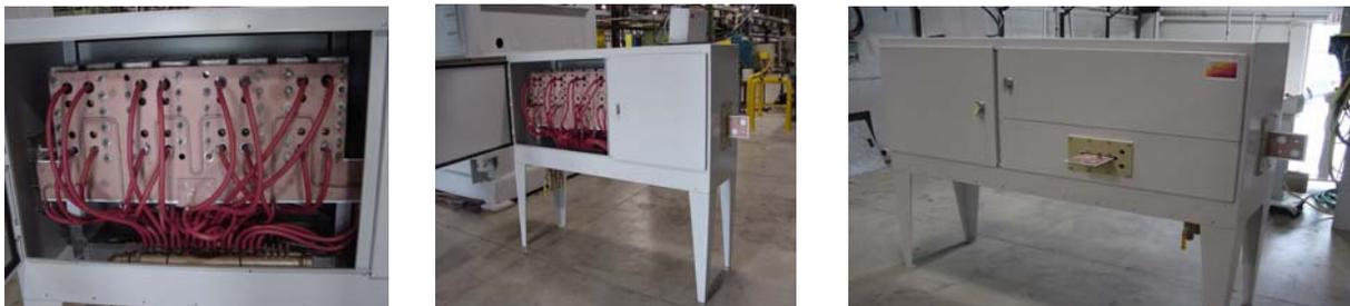
Figure 41. Tuning cabinet is completed allowing the proper voltage and capacitance for matching the coils designed to the power supply
