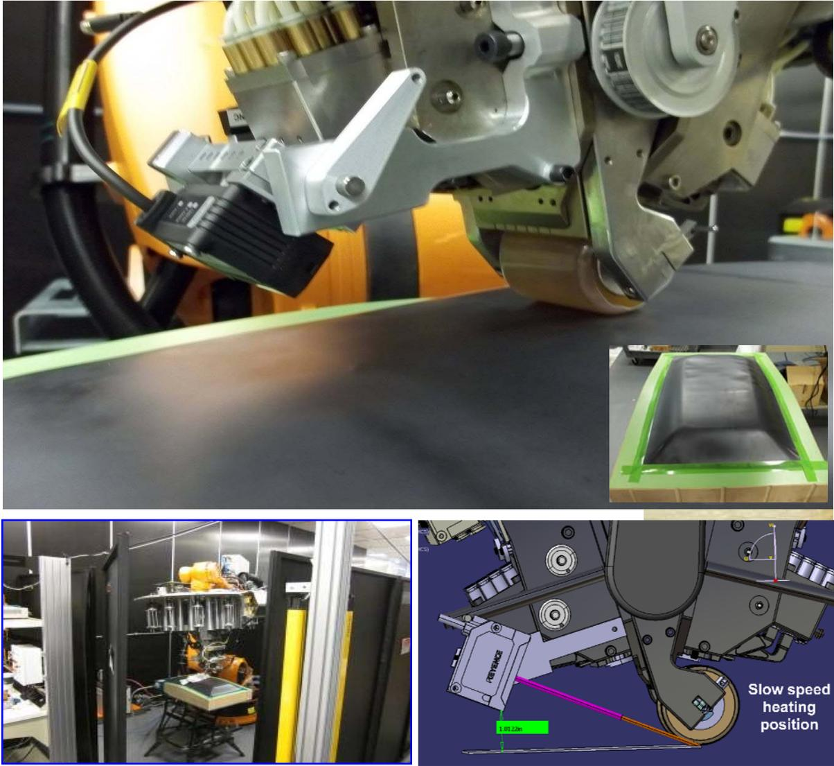
Figure 84. Pictures showing the integration of the laser system with a tow placement head for the application on slit thermoplastic tape
