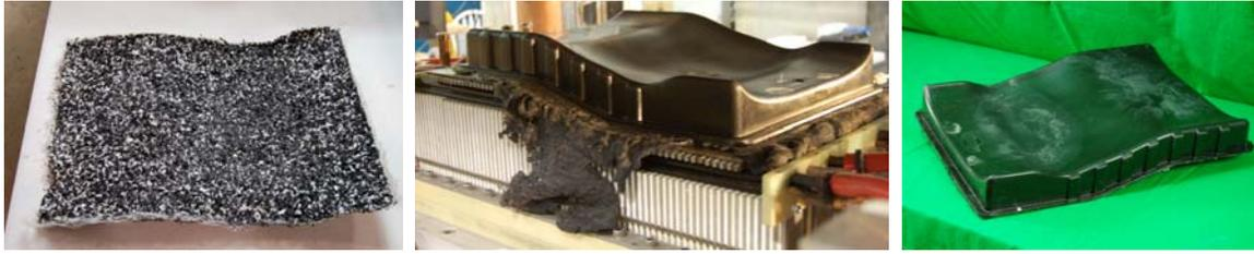
Figure 99. Incorporation of shredded fiberglass reinforce polypropylene material into the processing of an induction molded component
