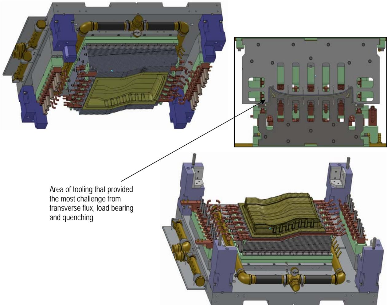
Figure 70. Induction molding tool design for the Ford seat pan is shown with the top and the bottom halves along with cross section of the tool running parallel to the stainless steel laminations
