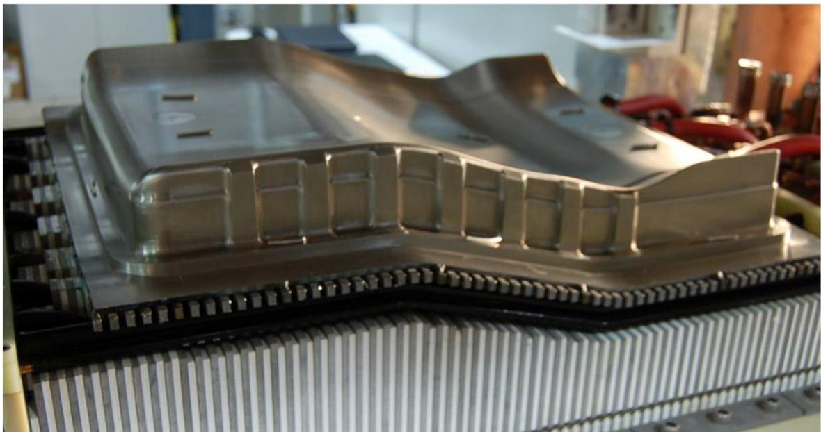
Figure 73. Complete bottom half of the Ford seat pan tool showing the detail of the machined susceptor
