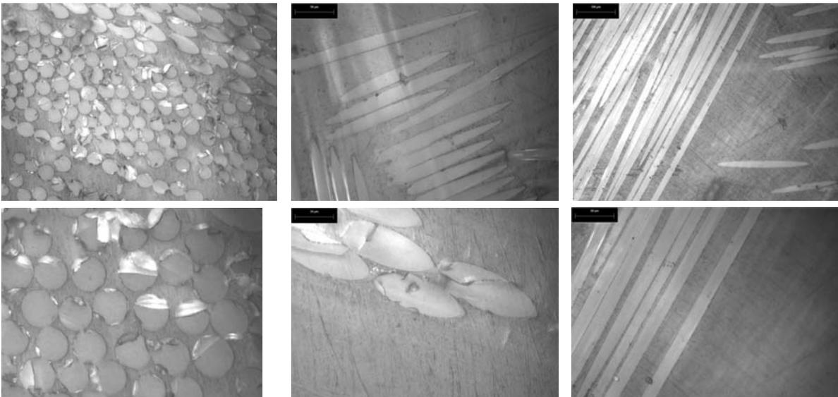
Figure 81. Pictures showing the typical microstructure of the induction molded Ford seat pan and depicting virtually no porosity
