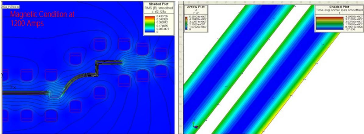
Figure 22. Boeing seat back with initial magnetic flux line shown when the smart susceptor is still non-magnetic on the left and the resulting current distribution (with currents either going into or out of the page) in each of the smart susceptor shells on the right
