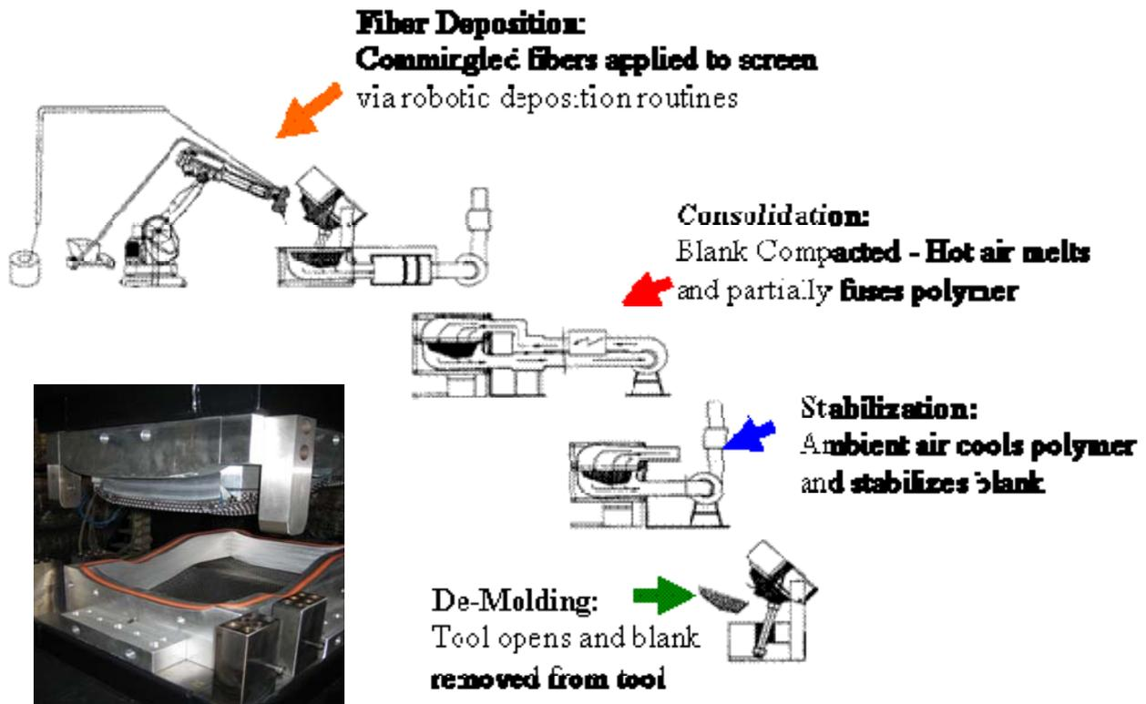
Figure 85. Process description for the Ford seat pan preform fabrication using a robotically manipulated chopper gun for spraying the fiberglass reinforce polypropylene
