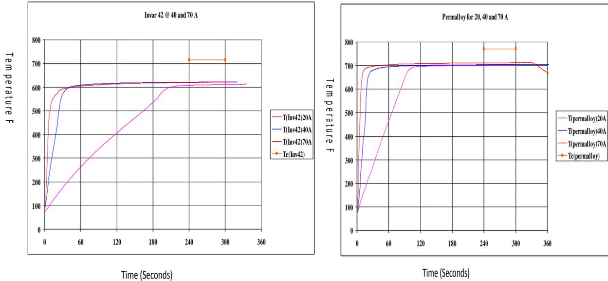
**Figure 6. Induction heating test results for Invar 42 smart susceptor on the left and for Moly-Permalloy on the right. Each figure shows the insensitivity of the smart susceptor leveling point to the applied current and the effectiveness of the thermal control even with constant current being applied throughout the test.**
