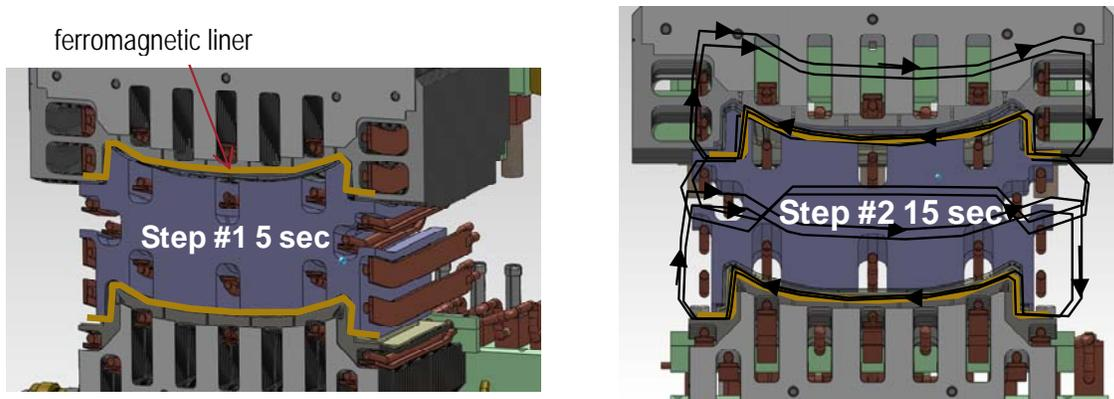
Figure 31. Depiction of smart susceptor preheating using tooling inserts with nonconductive ferromagnetic shells to reduce transverse flux issues allow very rapid preheating of the tool
