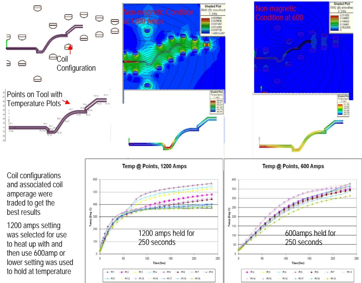
Coil configurations and associated coil amperage were traded to get the best results
