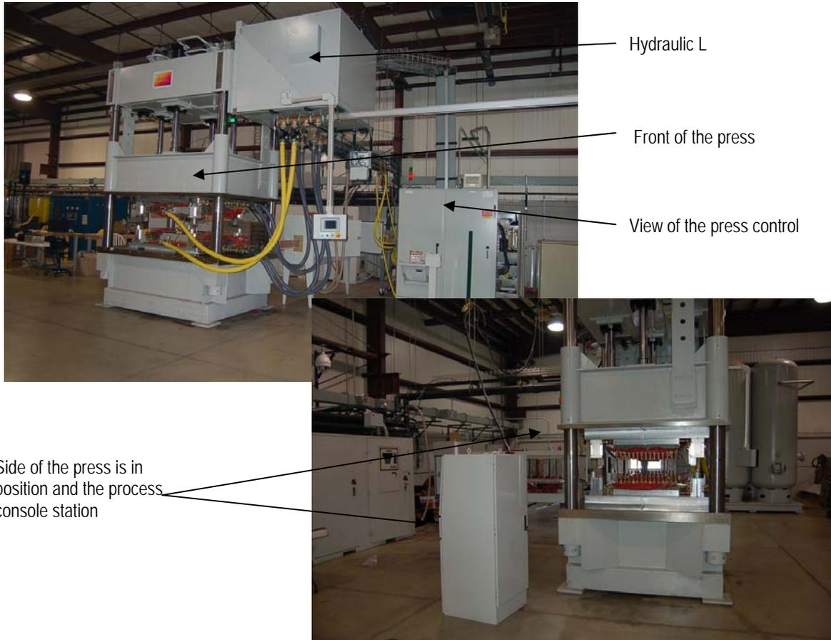
Figure 44. Completed, installed, and integrated induction consolidation/molding system ready to begin processing components
