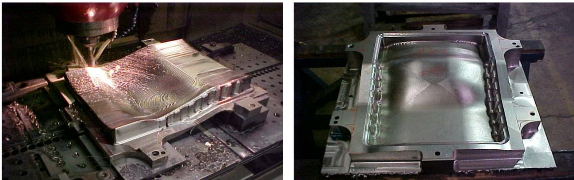
Figure 71. Machining of the smart susceptor shells from blocks of DK 510 alloy
