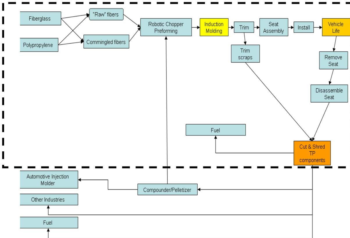
Figure 98. Indirect recycling stream outside automotive production boundary
