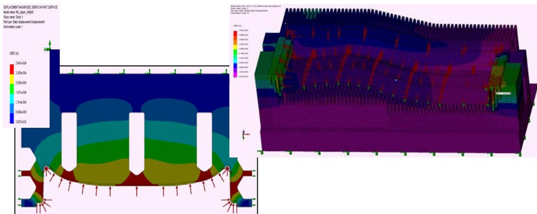
Figure 25. Stress analysis of the stainless steel laminations on the left and loading map of the smart susceptor on the right used to refine and optimize the tool design
