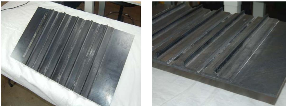
Figure 20. Photo of the completed integrated/welded structural panel
