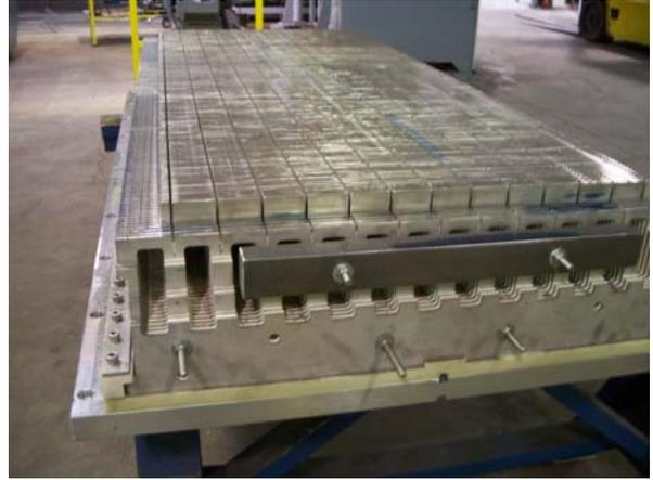
Figure 60. Trimmed stainless steel laminations on the left and subsequent assembly of the laminations making up the tool body for the Vestas tool on the right
