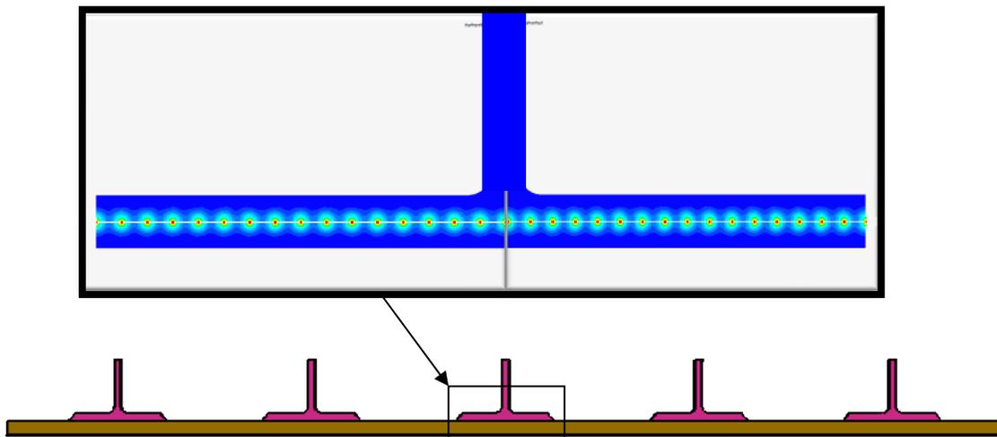
Figure 14. Depiction of the weld joint for the demonstration panel that was fabricated - note the location of the smart susceptors in the weld joint.
