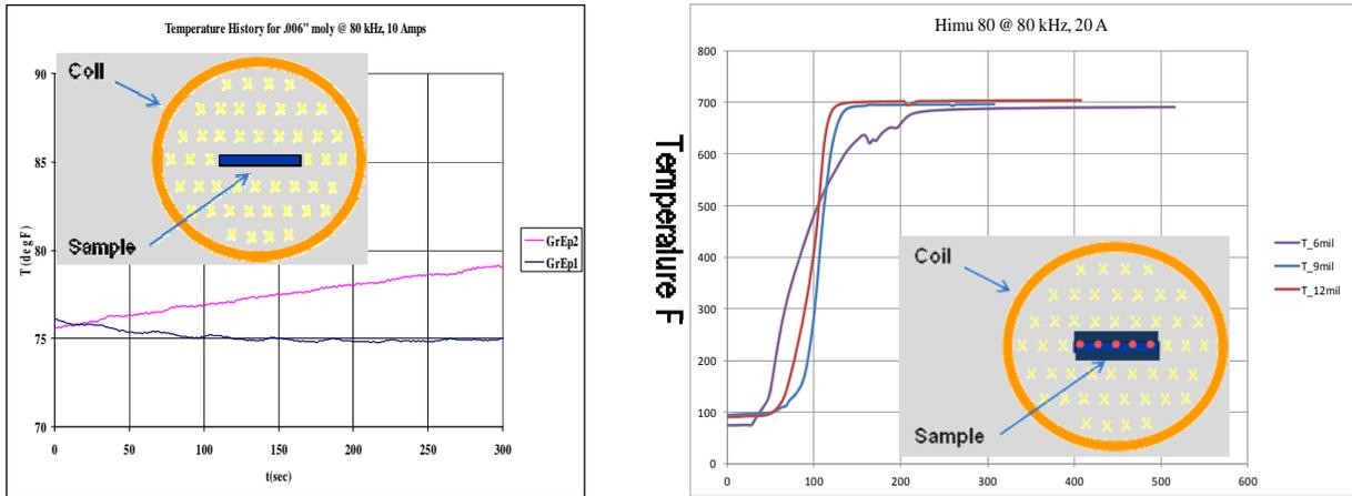
Figure 13. Graph on the left shows the heating behavior of the graphite reinforce composite material while the graph on the right shows the heating behavior of the composite with HyMu 80 smart susceptor wires imbedded in it.
