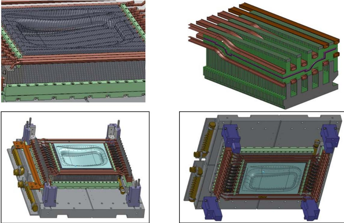
Figure 45. Boeing seatback tool design showing the induction coil, the stainless steel tool body laminations, the smart susceptor shells, and the die shoes for easy handling
