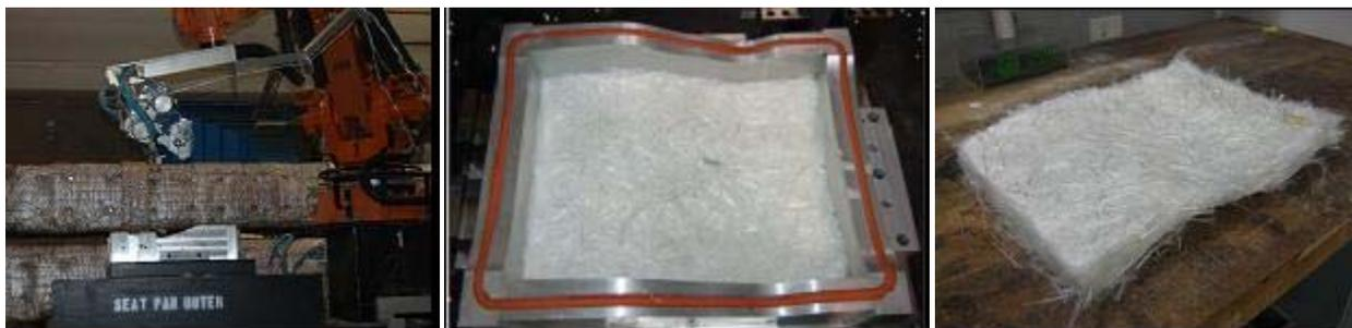
Figure 86. Pictures of the preform tooling, the robotically manipulated chopper gun, and a stack of completed preforms
