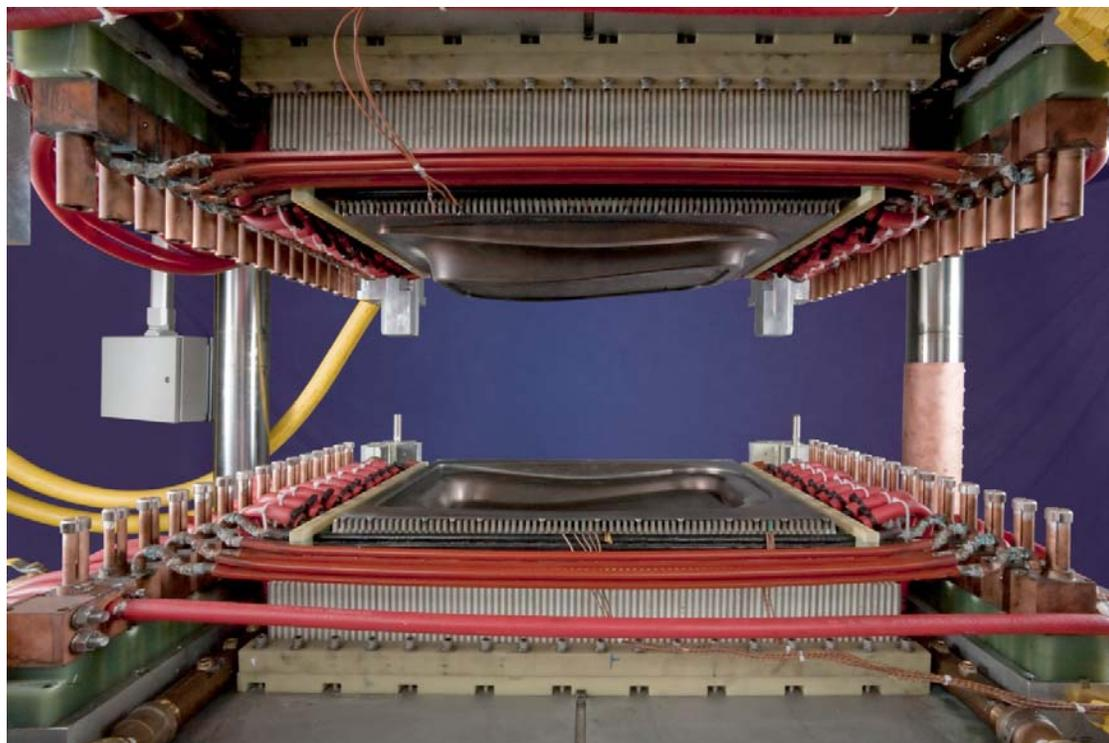
Figure 51. Front view of the completed Boeing seatback tool installed in the induction press and ready for molding
