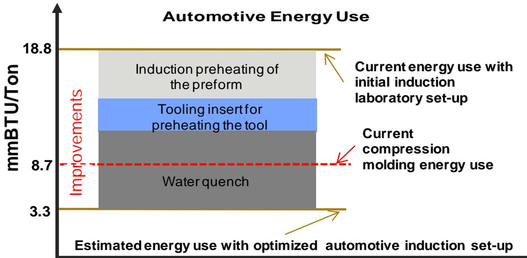
Figure 94. Comparison of the energy used for by the current automotive resistively heated compression system and the current induction laboratory system and the potential energy efficiency of an optimized induction processing system
