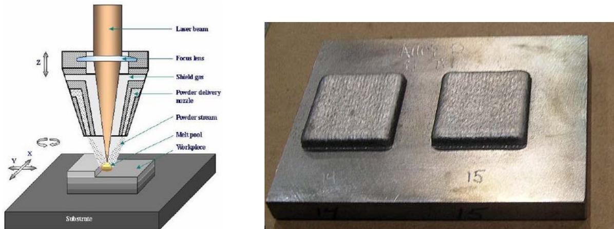
Figure 12. Depiction of the laser engineered net shaping (LENS) process in operation and a picture of the one of the custom alloy samples produced for evaluation
