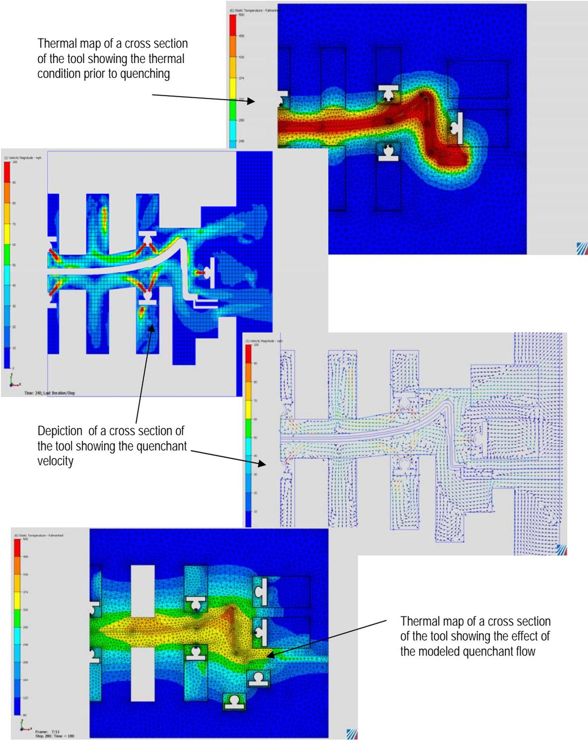
Figure 26. Depictions showing the utilization of the thermal and CFD analysis of the Ford seat pan tool to refine the placement of the active cooling medium for quenching
