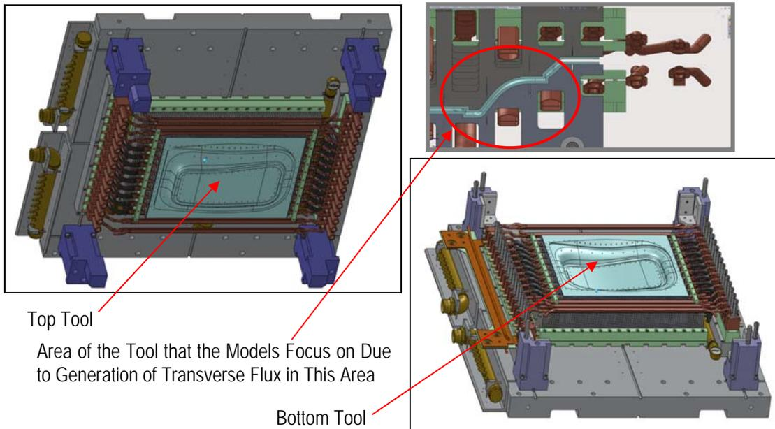
Figure 21. Boeing seat back tool design using the smart susceptors “shells” as the tool faces and the solenoidal shaped coil that surrounds these shells
