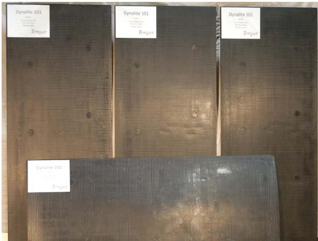
Figure 68. Photo of the fiberglass fabric reinforced nylon6-6 panels fabricated and ready for evaluation
