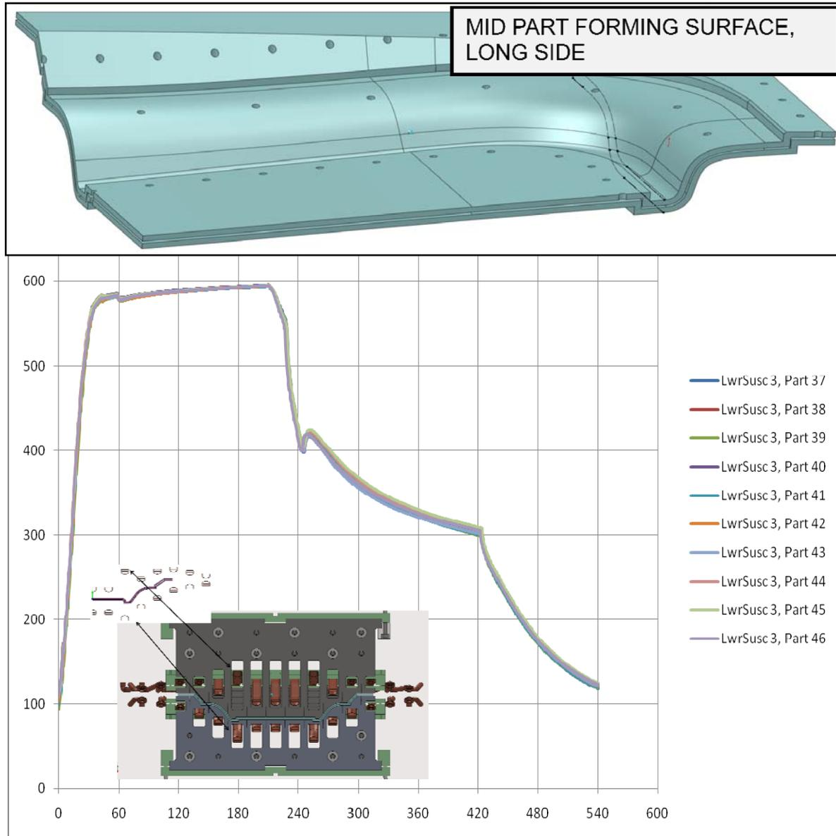
Figure 55. Graph showing the thermal repeatability of the process with the same spot on the tool over a 10 part run with almost the exact profile on each processing run
