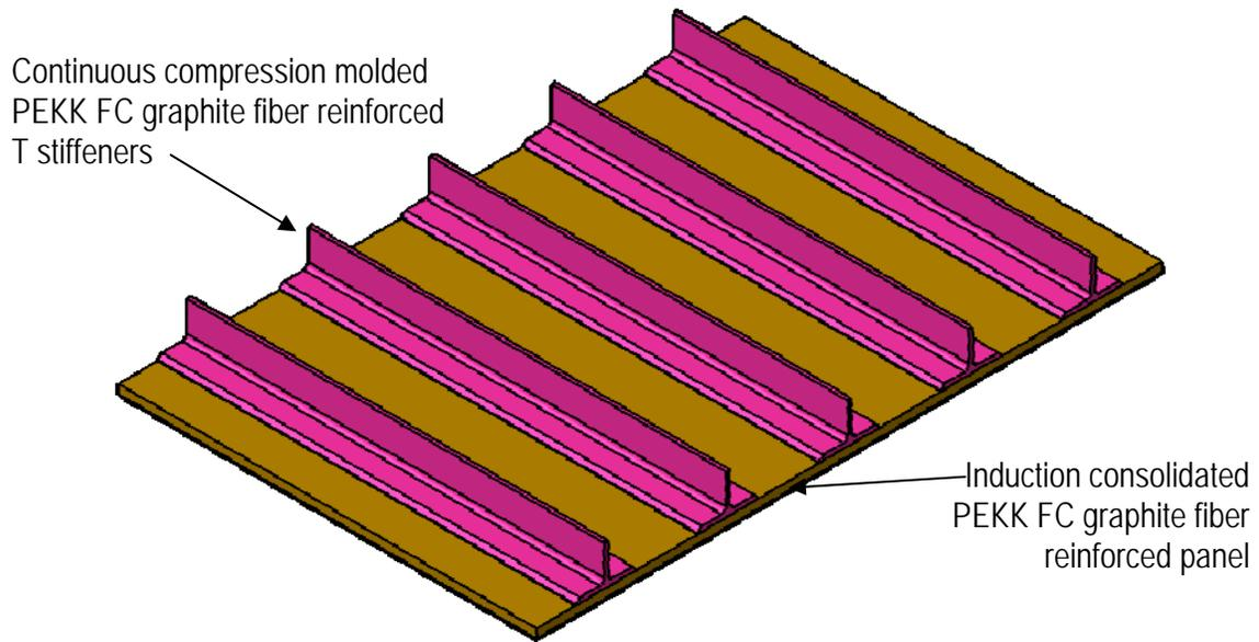
Figure 15. Depiction of the demonstration panel that was fabricated with 5 T stiffeners welded to the flat panel
