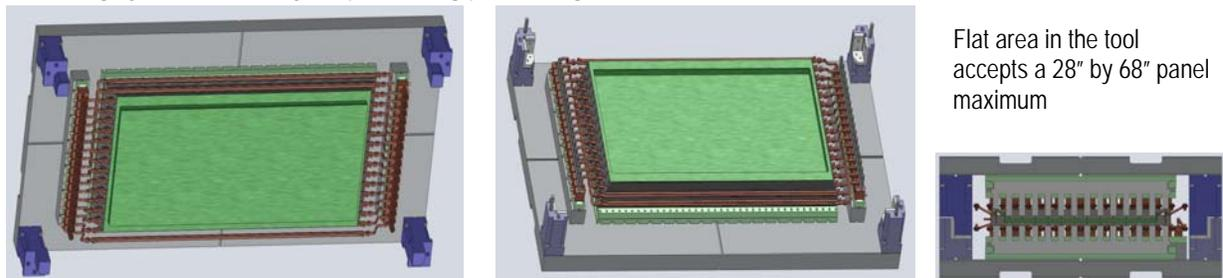
Figure 59. Vestas flat panel tooling design
