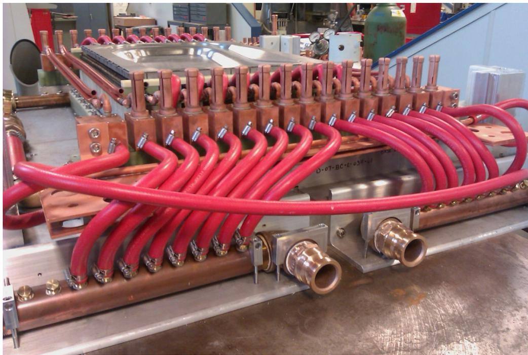
Figure 50. Side view of the completed lower tool half showing the quick disconnect for the cooling water feeding each of the induction coil turns
