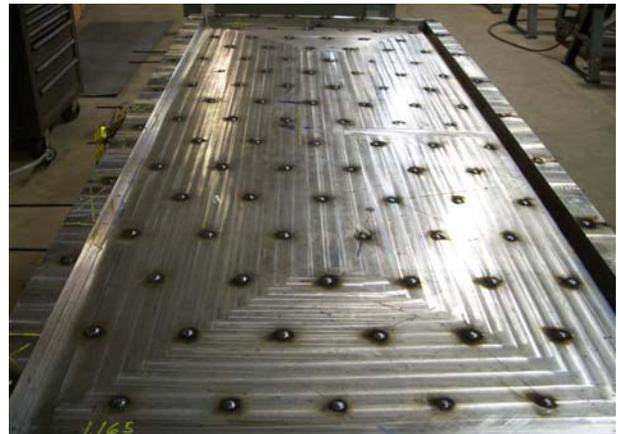
Figure 61. Machined smart susceptor being loaded onto the assembled laminations and then the subsequent tacking of the smart susceptor to the laminations
