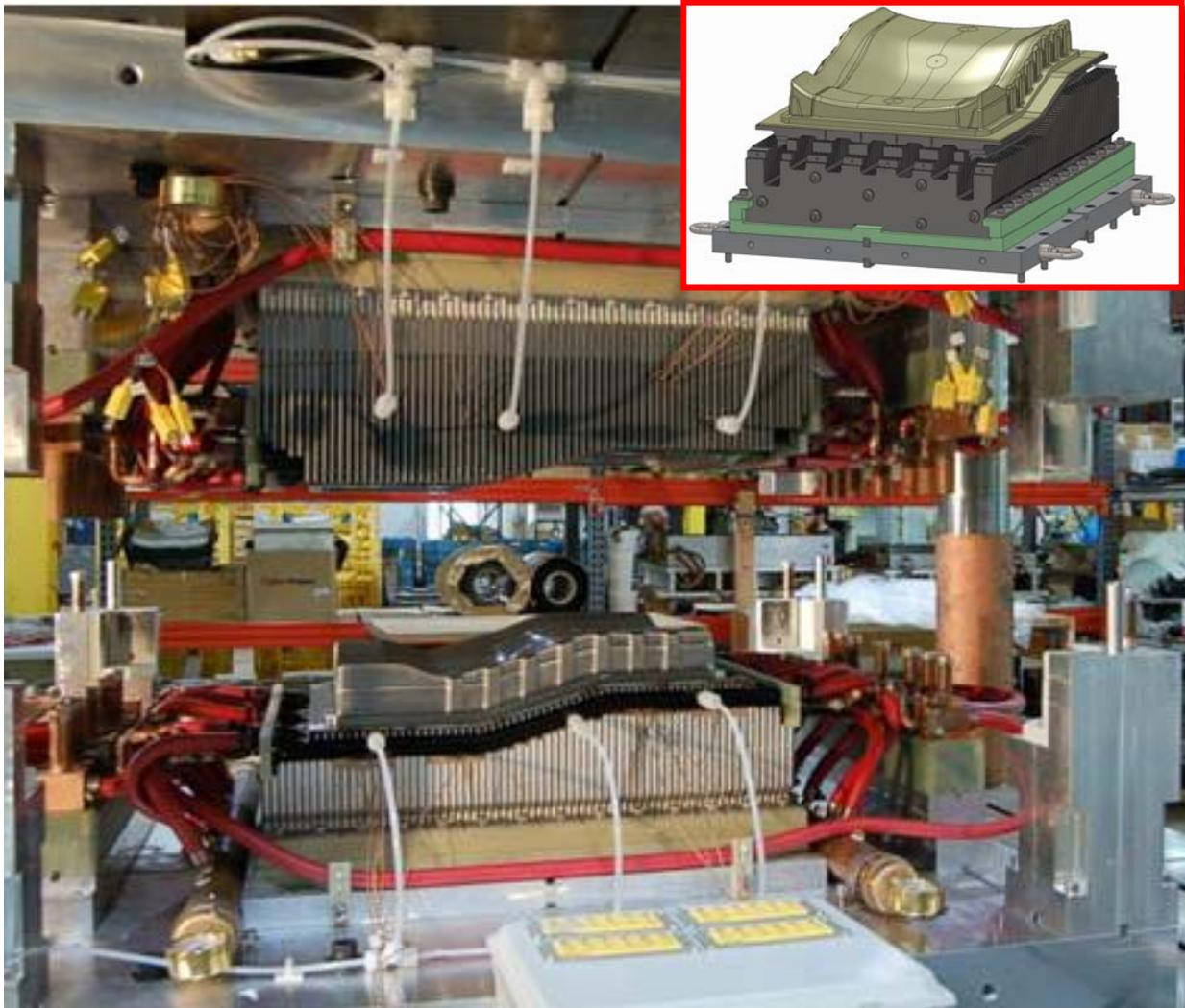
Figure 74. Ford set pan tool installed in the induction processing system and ready to begin part molding
