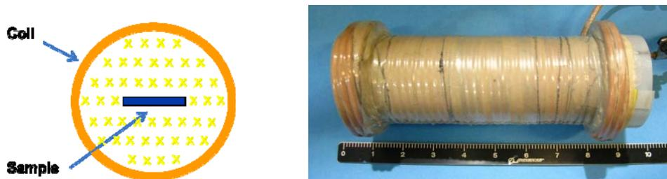
Figure 8. Test coil used for evaluation of candidate smart susceptor alloys.
