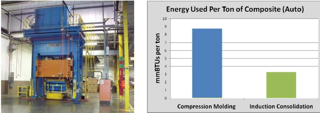
Figure 89. Comparison on the energy use by the standard automotive composite processing system (resistively heated compression molding press) and the induction consolidation process
