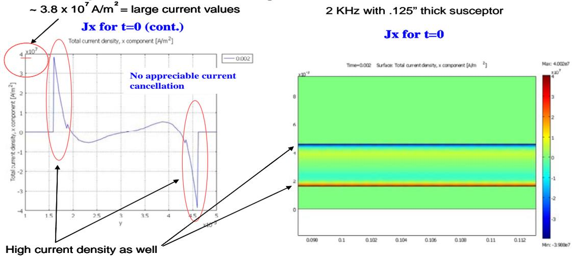
Figure 3. Depictions of the induced current distributions in the smart susceptor, with the magnetic state depicted on the left and the non-magnetic state shown on the right
