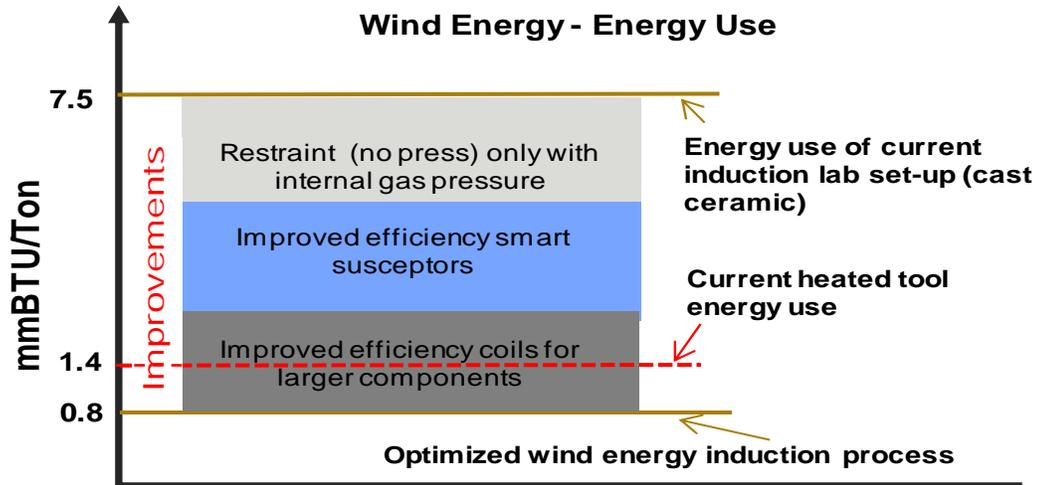
Figure 93. Comparison of the energy used for by the current wind energy self heated tooling system and the current induction laboratory system and the potential energy efficiency of an optimized induction processing system
