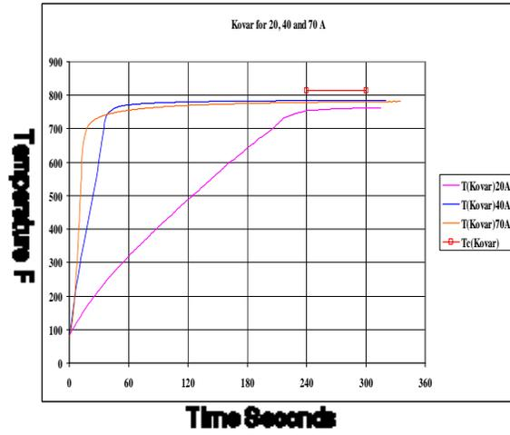
Figure 9. Thermal leveling test results for Moly-Permalloy (HyMu80) on the left and Kovar on the right
