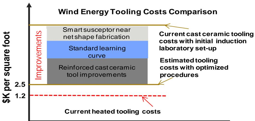
Figure 102. Chart depicting the current cost of the induction consolidation tooling to the existing self heated tooling cost plus the estimated tool cost savings available for the optimized induction process
