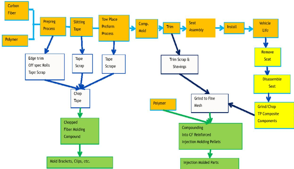
Figure 95. Aircraft Seat Back Life Cycle Flow Diagram with Recycle Streams
