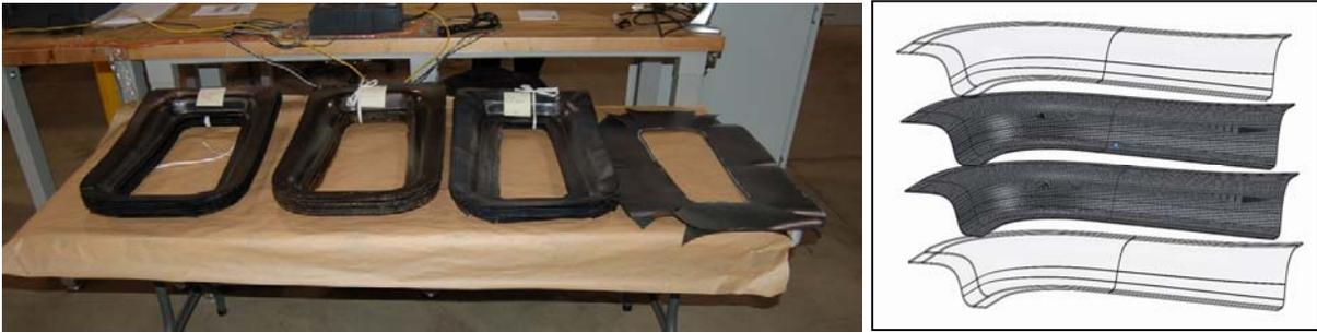
Figure 53. Picture of the graphite fiber reinforced PEKK DS fabric preforms ready for consolidation on the right side of the picture along with the consolidated components on the left side of the picture
