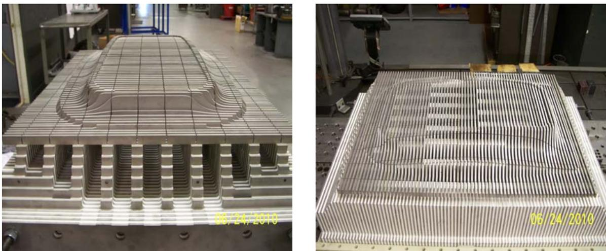
Figure 46. Picture of the assembled stainless steel tool body laminations for both the upper tool and the lower tool halves
