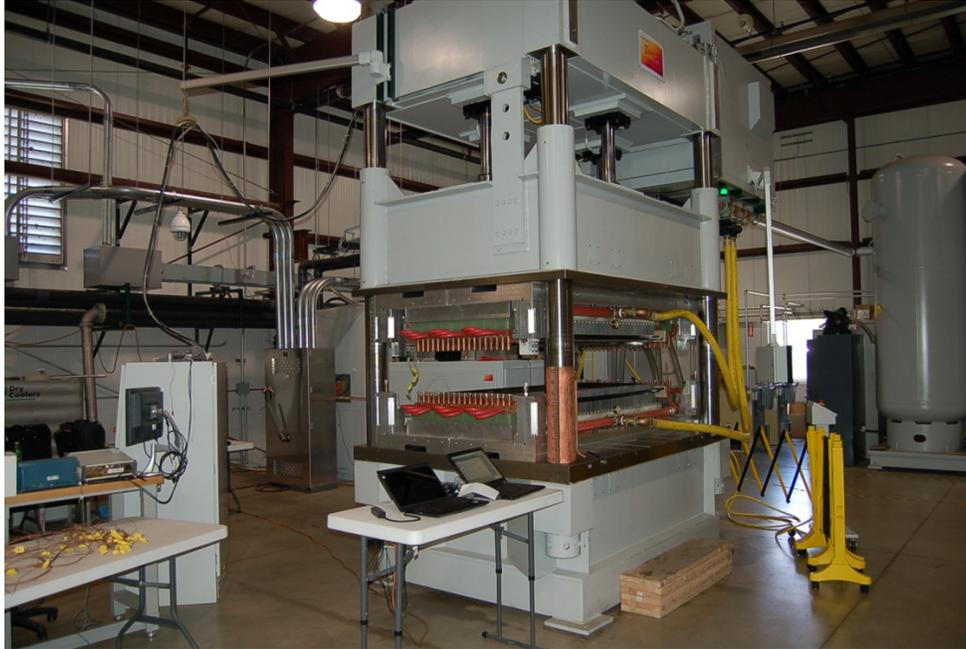
Figure 63. Picture showing the completed Vestas tool installed in the induction processing system and ready to begin molding trials
