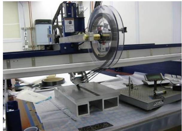
Figure 82. 2-axis initial laser set-up to demonstrate the ability to effectively tack down the thermoplastic prepreg tape
