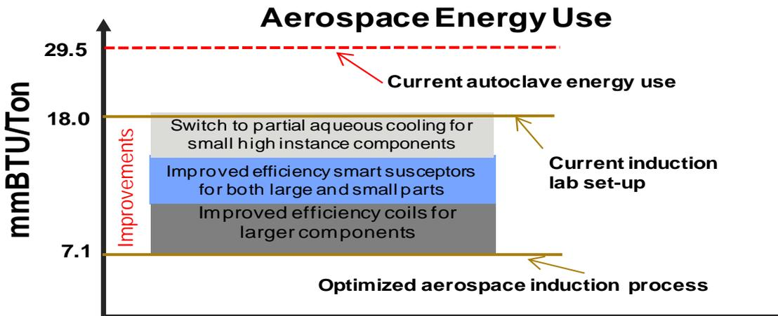
Figure 92. Comparison of the energy used for by the current aerospace autoclave system and the current induction laboratory system and the potential energy efficiency of an optimized induction processing system
