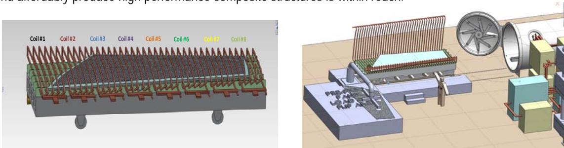
Figure 29. Depiction of a series/parallel coil for consolidating a large aircraft skin section utilizing a pneumatic pressurization facility for application of consolidation pressures
