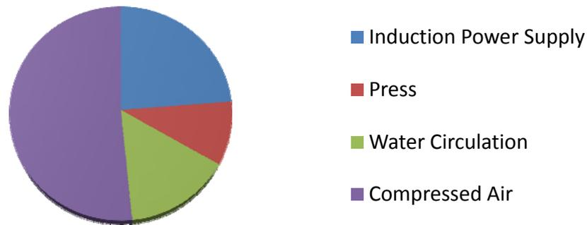
Figure 91. A pie chart showing the contributions of each of the 4 main systems that comprise the induction processing facility
