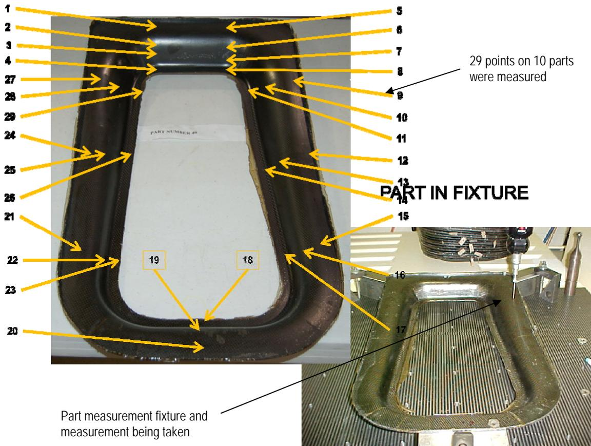
Figure 57. Picture on the left shows the points measured during the dimensional evaluation using a coordinate measurement machine (CMM) with a photo of the part set up shown on the right
