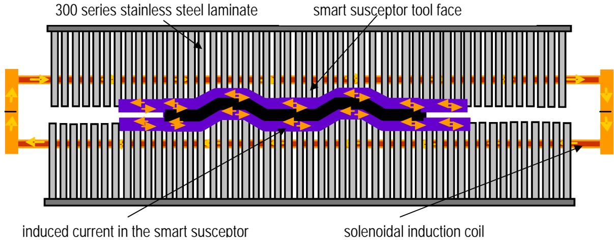
Figure 1. Typical tooling construction concept associated with the tool designs being developed
