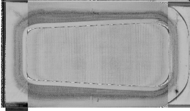
Figure 56. Typical ultrasonic inspection results for the induction consolidated Boeing seat back part showing acceptable overall quality
