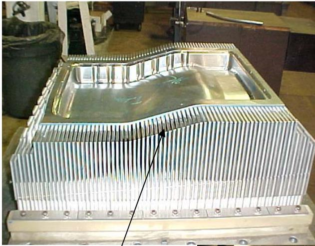
Additional lamination extended out from the susceptor to resist the load pushing out from the sides of the component during molding
