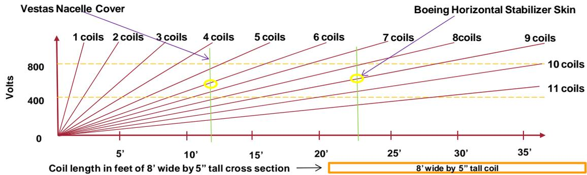
Figure 27. Graph showing the required number of coils connected in parallel to keep the required circuit voltage at practical levels (between 400 and 800 volts) for a given length of coil having 8 foot by 5 inch cross sectional area
