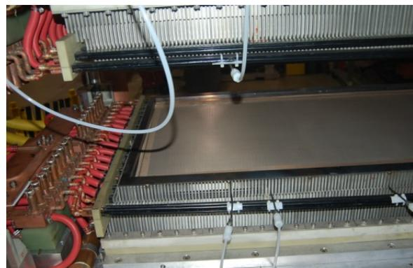
Figure 64. Pictures showing layers of the fiberglass/nylon fabric placed in the part molding cavity and the subsequent lay-up in the tool ready for consolidation
