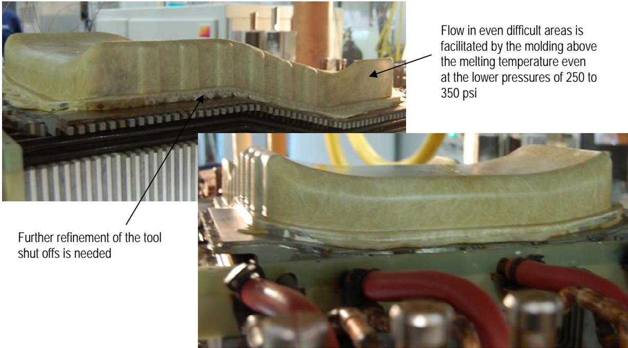
Figure 78. Initial as molded Ford seat pan component showing the complete flow of the material in all areas of the tool
