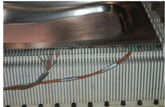
Figure 47. Side view of the stainless steel tool body laminations assembled with the smart susceptor shells tack welded on and subsequently finished machined
