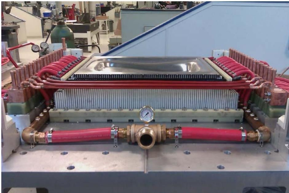
Figure 49. Front view of the completed lower tool half showing the quick disconnect for the quenching air feeding the individual quenching tubes
