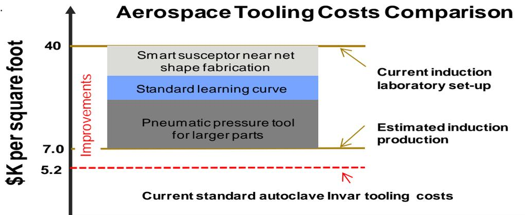
Figure 100. Chart depicting the current cost of the induction consolidation tooling to the existing autoclave tooling cost plus the estimated tool cost for the optimized induction process
