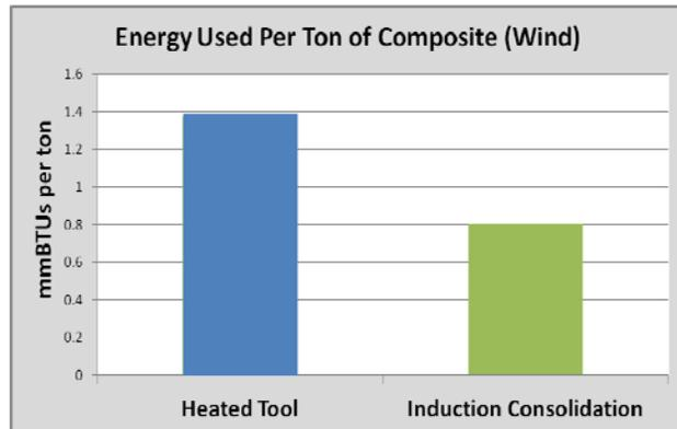
Figure 88. Comparison on the energy use by the standard wind energy composite processing system (convectively heated tool) and the induction consolidation process
