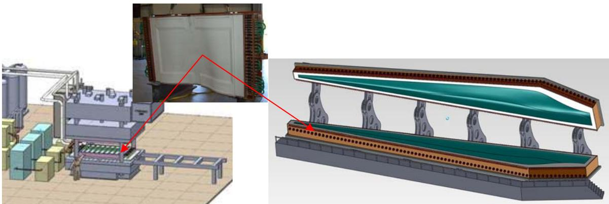
Figure 30. Depiction of the large induction consolidation facility for processing nacelle panels on the left and blade skins on the right
