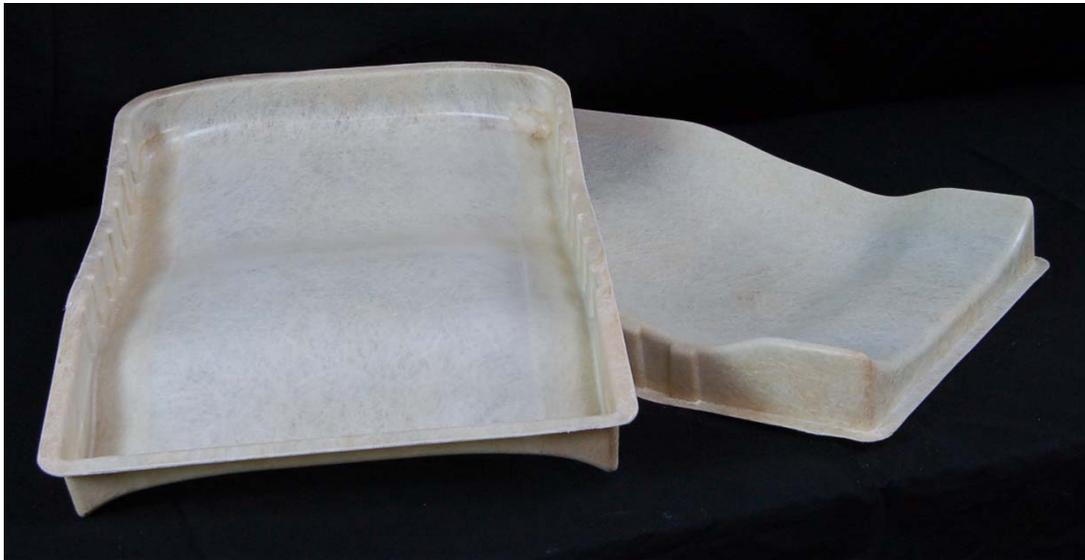
Figure 79. Resulting induction molded Ford seat pan components
