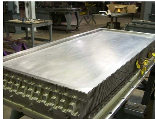
Figure 62. Final machining of the susceptor after tacking to the laminations on the left and then the completed tooling insert on the right
