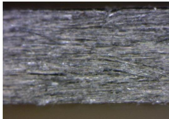
Figure 83. Resulting tacked material showed no damage from the laser due to the very controlled types of lasers and a stable lay-up of material
