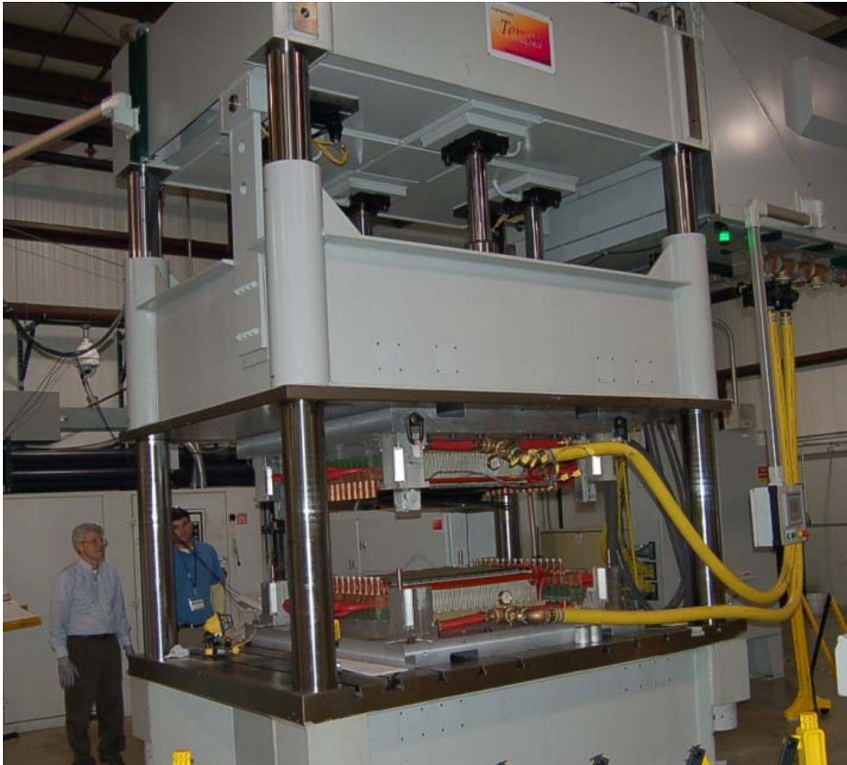
Figure 52. View of the completed Boeing seatback tool installed in the completed processing system along with the attachment of the air quenching yellow lines to the quick disconnect fittings
