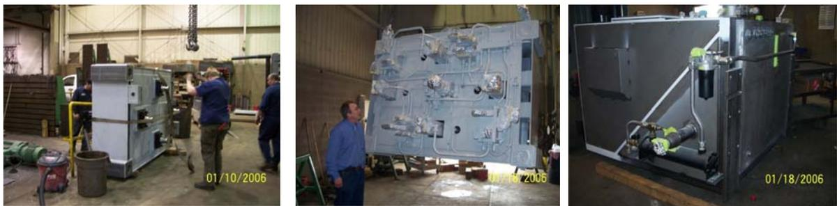
Figure 38. Pictures of the installation of the new hydraulic cylinders/system in the redesigned press
