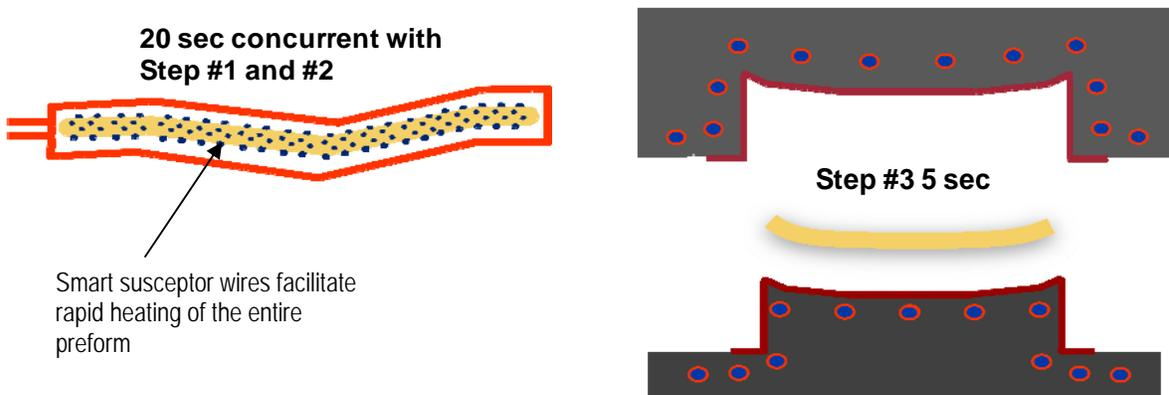
Figure 32. Depiction of a system for rapidly preheating of the preform on the left using smart susceptor wires to quickly heat the preform and then the preheated preform is loaded into the preheated tool
