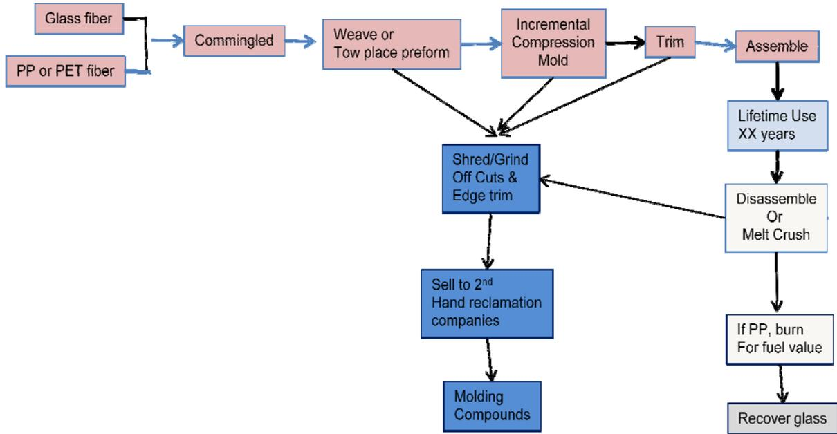
Figure 96. Wind Energy Material Life Flow Diagram with Recycle Streams
