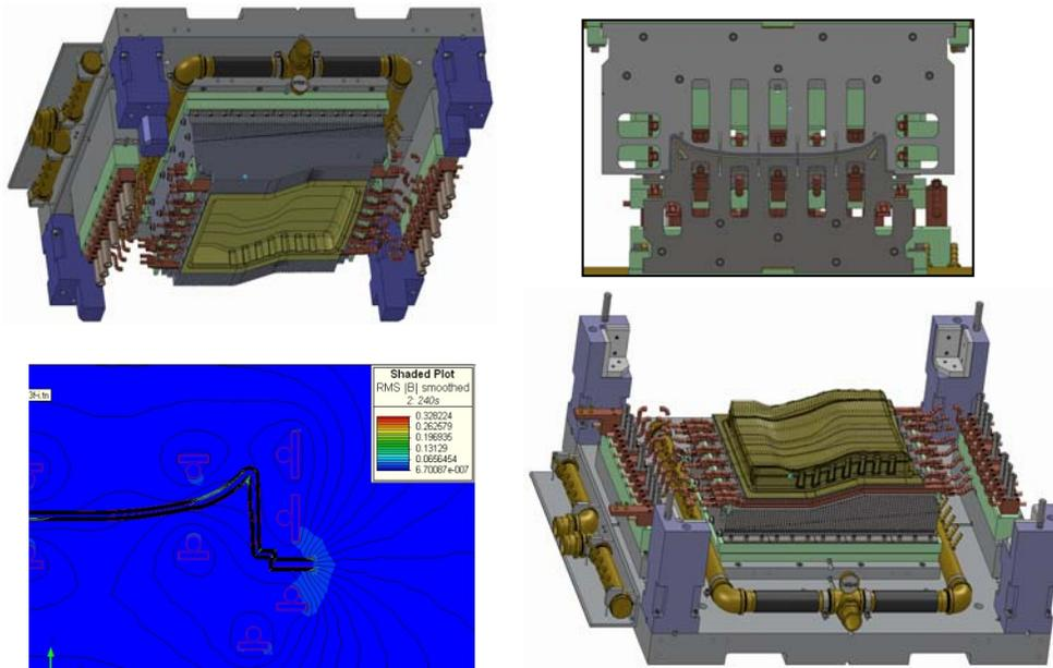
Figure 24. Depictions of the Ford tooling design and the associated electromagnetic analysis
