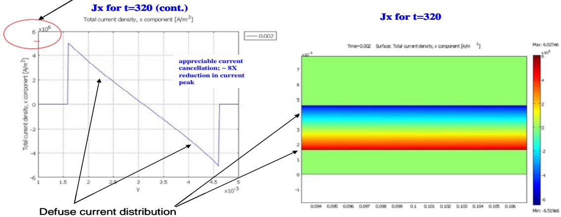
Figure 4. Depictions of the induced current distributions in the smart susceptor, with the magnetic state shown on the left and the non-magnetic state shown on the right
