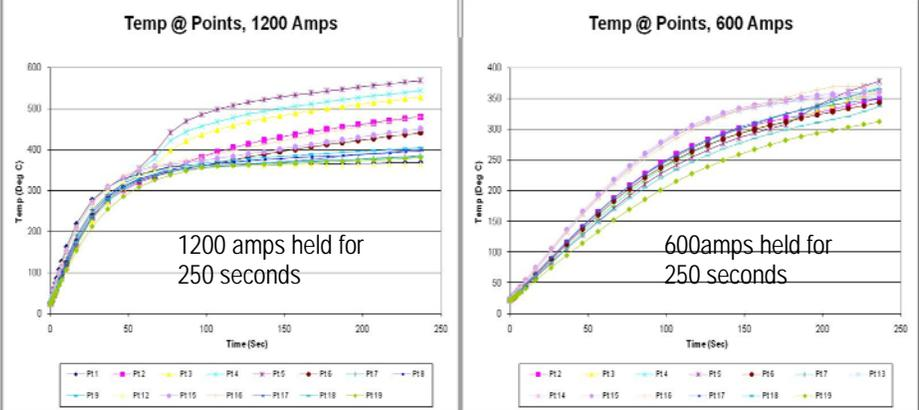
Figure 23. Electromagnetic analysis with resulting thermal condition showing the results of lowering the amperage once the smart susceptor shells reach the leveling temperature
