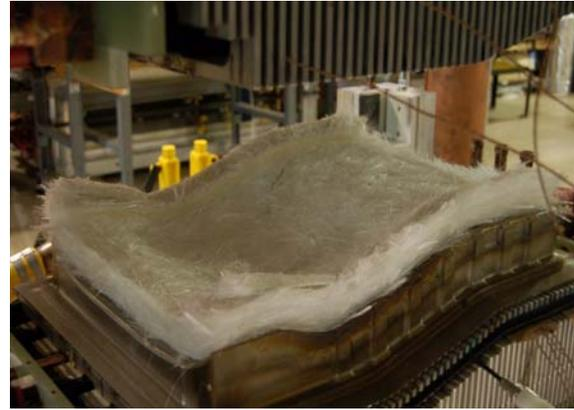
Figure 75. Two pictures of the robotically sprayed chopped fiberglass fiber and polypropylene rovings making up the Ford seatpan preforms ready for induction molding
