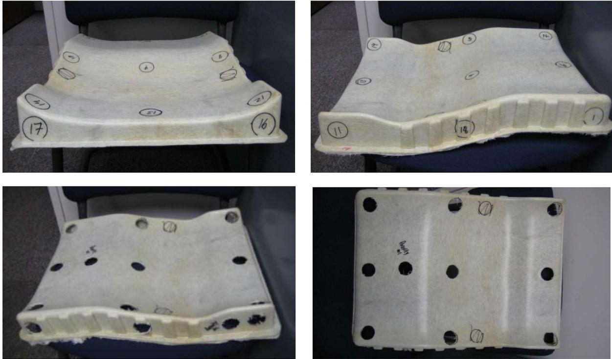
Figure 80. Candidate induction molded seat pan with sections identified for evaluation via microscopy (top pictures) and the part with the evaluation samples subsequently removed (bottom pictures)
