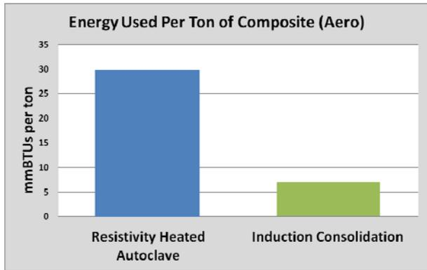
Figure 87. Comparison on the energy use by the standard aerospace composite processing system (resistively heated autoclave) and the induction consolidation process
