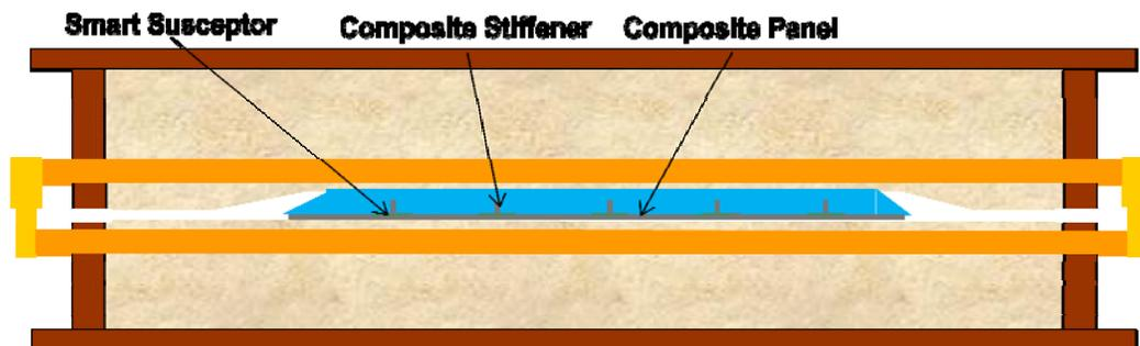
Figure 17. Depiction of the elastomeric caul holding the T stiffeners to the flat panel via pressure from the ceramic-tool/press during the welding process
