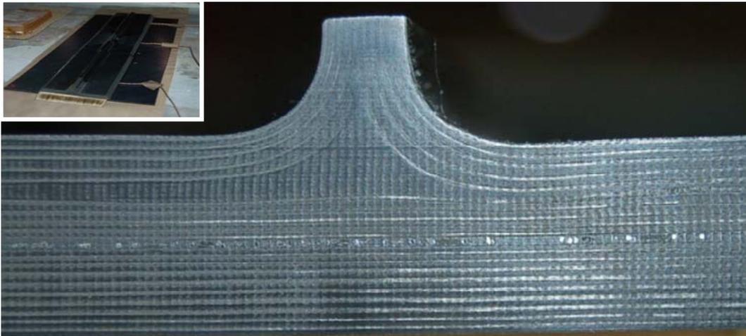
Figure 19. A close-up photograph of a typical joint in the welded panel
