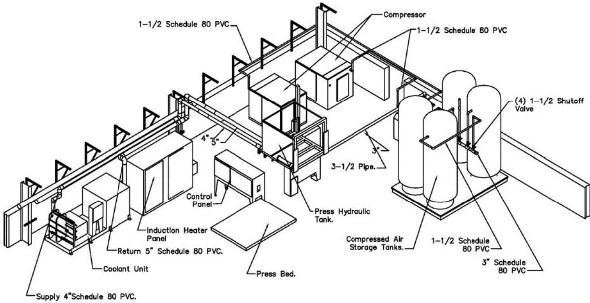
Figure 42. Induction processing system schematic showing the elements of the process plus pictures of the installed air quenching pressurized tanks
