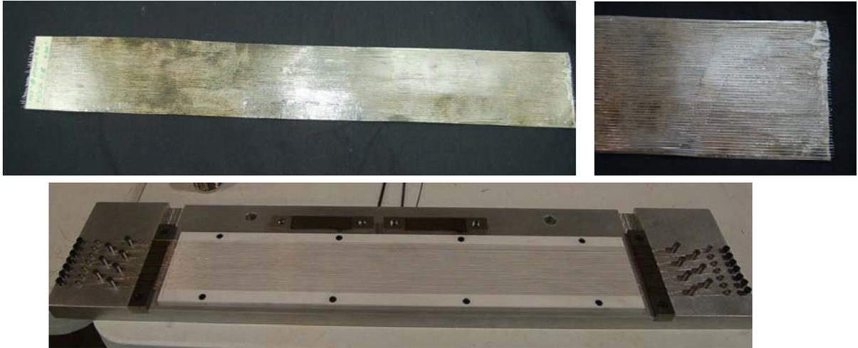
Figure 18. Photos of the tool for imbedding the smart susceptor wires in the thermoplastic resin and the strip of material produced
