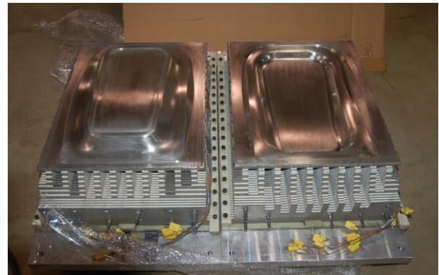
Figure 48. Side view of the stainless steel tool body laminations assembled with the smart susceptor shells tack welded on and subsequently finished machined
