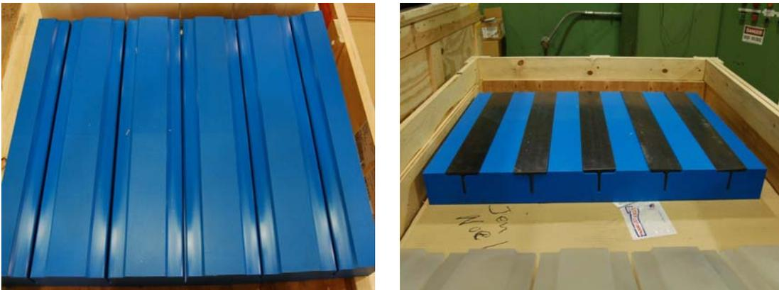
Figure 16. Photo of the elastomeric caul that will hold the T stiffeners in place and provide the pressure to hold them in intimate contact during the welding process
