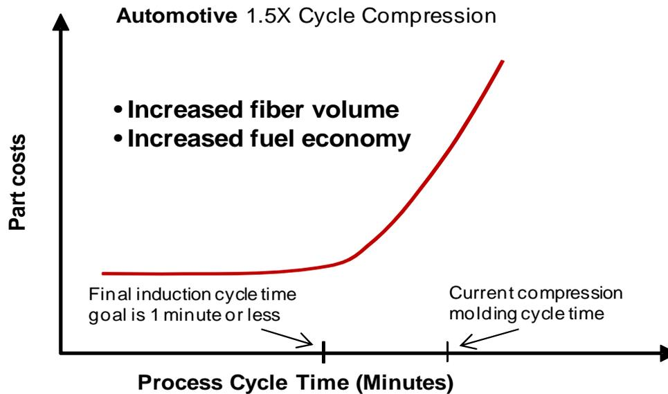
Figure 105. Depiction of the effect of a one minute induction processing cycle goal to the automotive part costs
